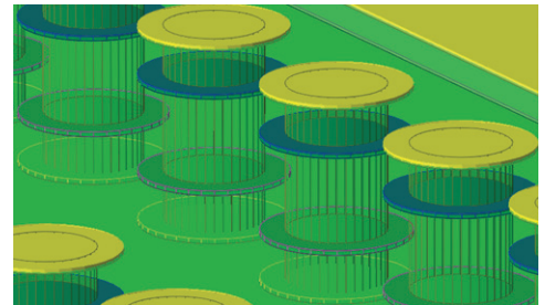
Proper via modeling is a critical component to accurate PCB simulations. Microwave Office thru vias showed in the layout view.
